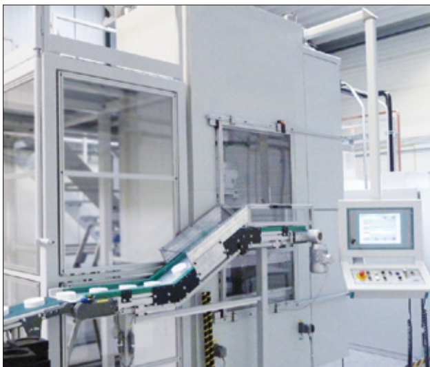
By using what is probably the most modern press in the dental field, WIELAND produces blanks of outstanding quality. The extremely high-pressure used ensures that the powder is highly compacted and homogeneous.
